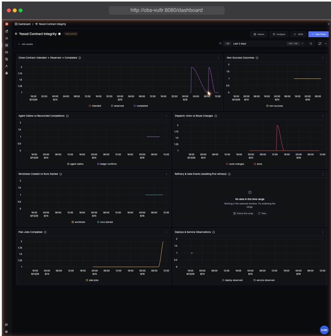
Figure 11.2.: The Contract Integrity dashboard: every panel pairs an intent with its confirmation.
